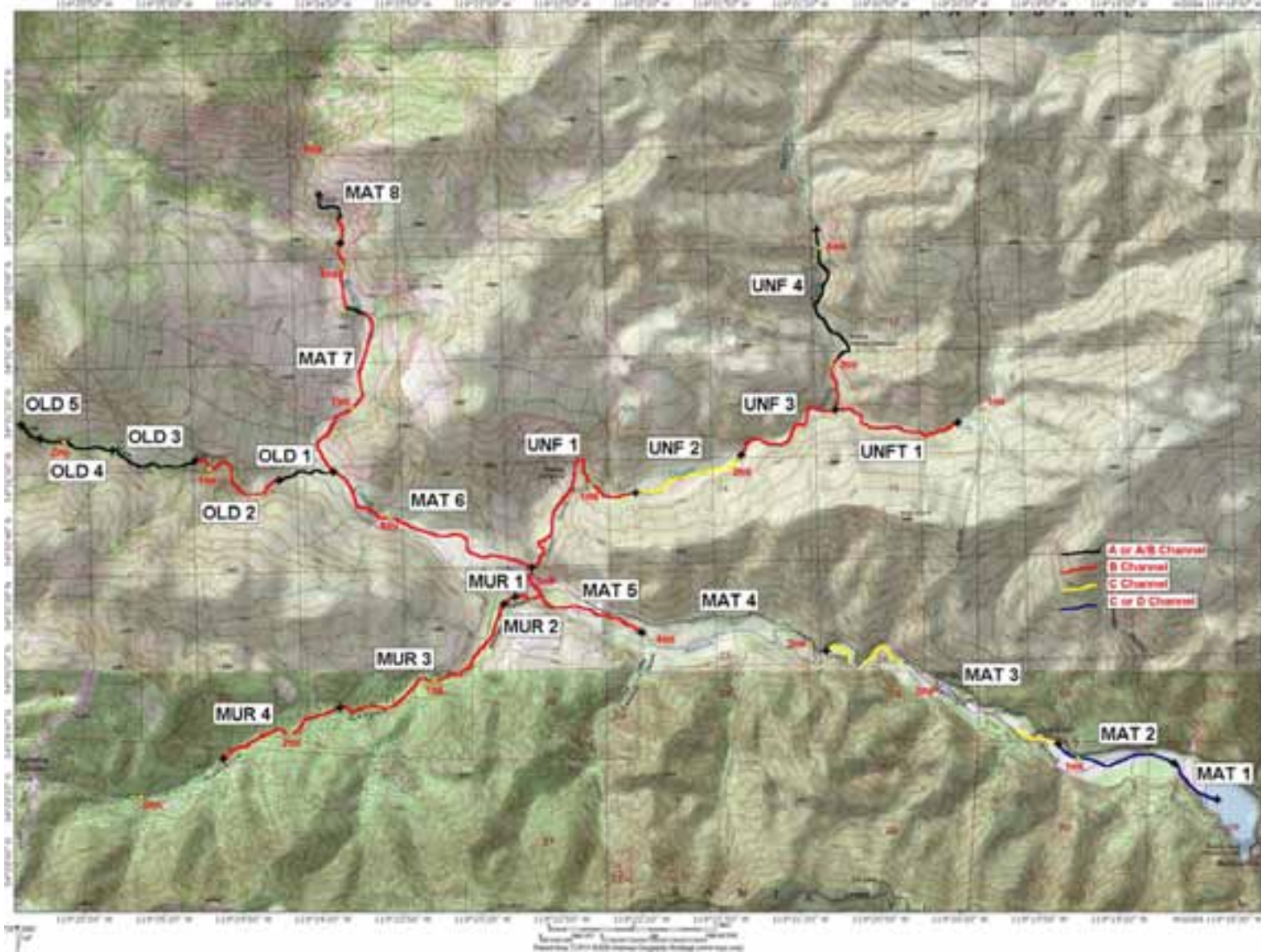
Figure 4. Map of the upper Matilija Basin showing reach boundaries and dominant channel types (colored lines). Channels not outlined were not mapped.
